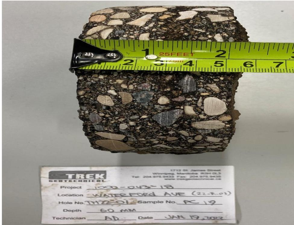
Photo 1: Pavement Core Sample at Test Hole TH22-01
