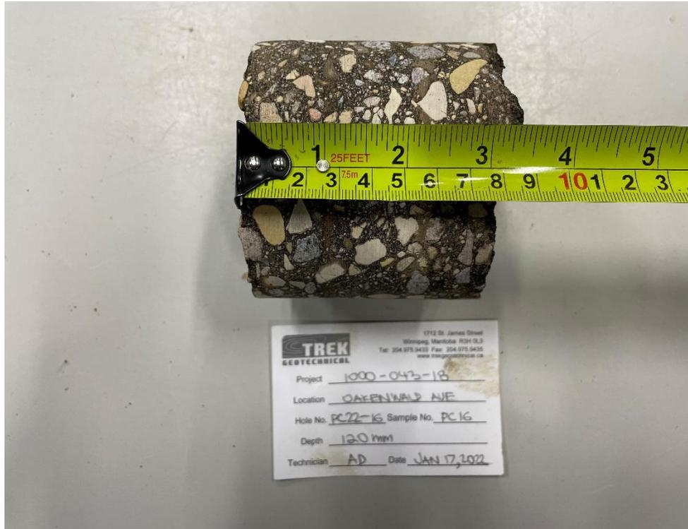
Photo 7: Pavement Core Sample at PC22-16
