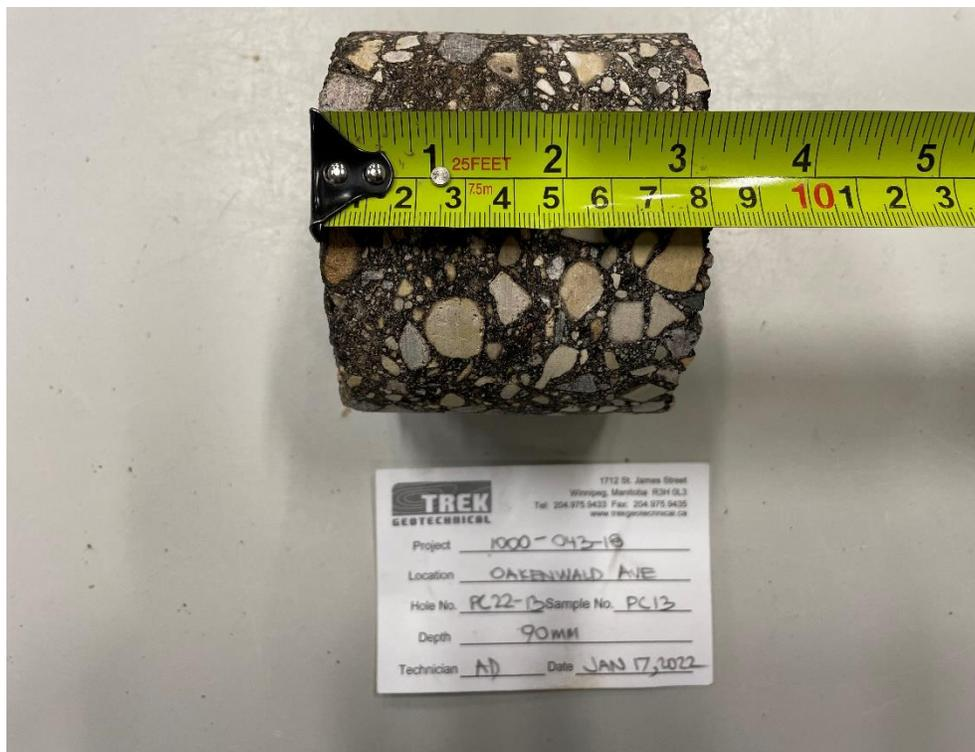
Photo 4: Pavement Core Sample at PC22-13
