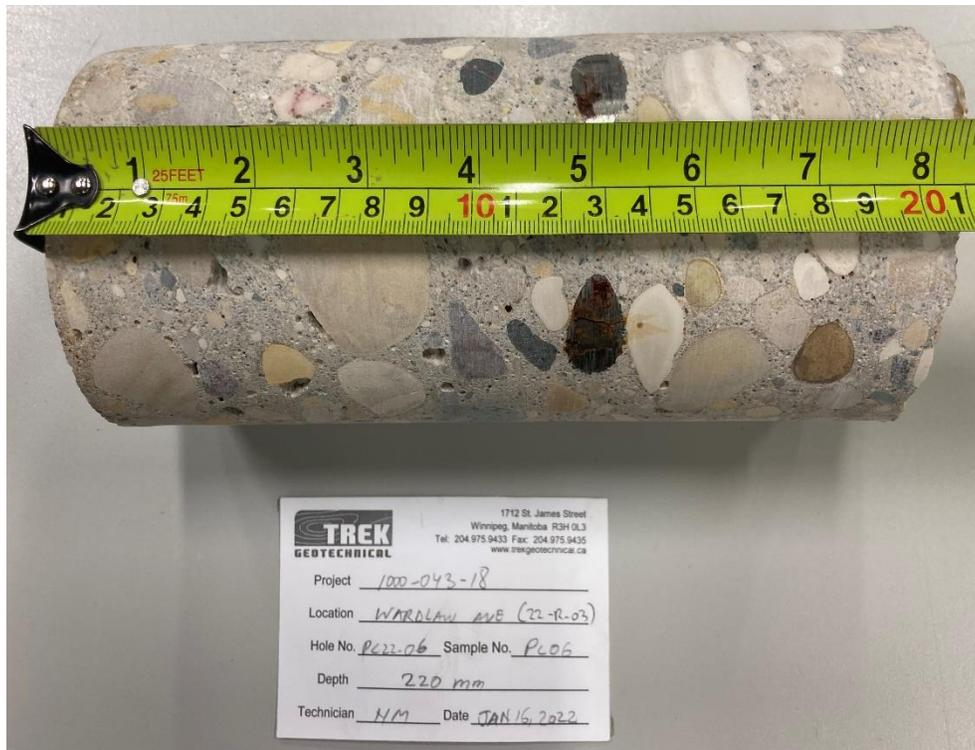
Photo 2: Pavement Core Sample at PC22-06
