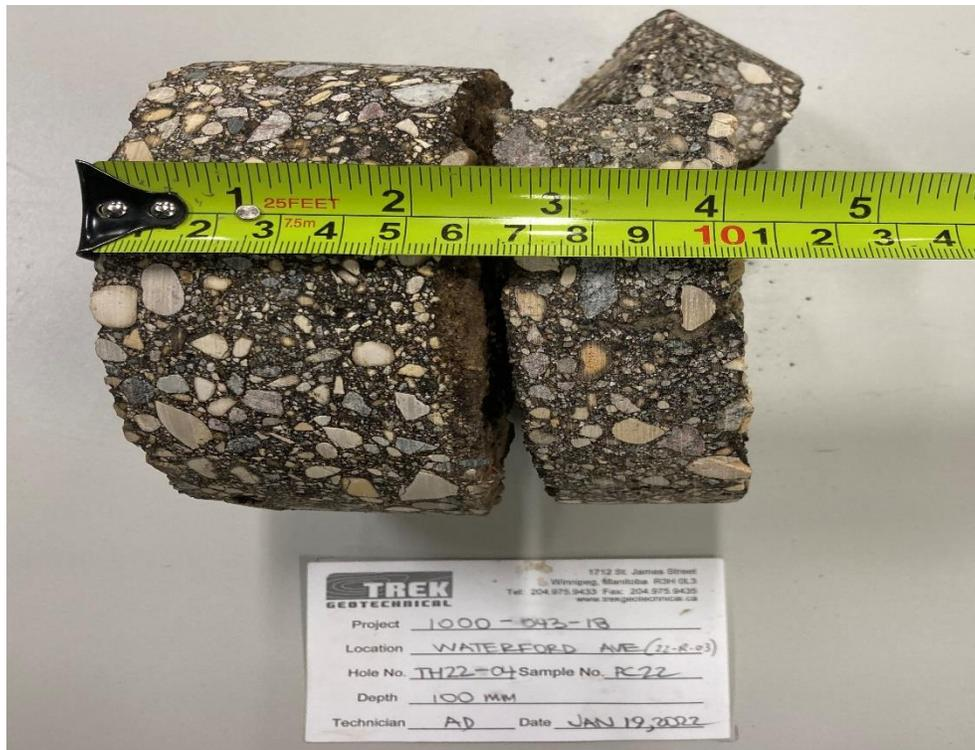
Photo 4: Pavement Core Sample at Test Hole TH22-04
