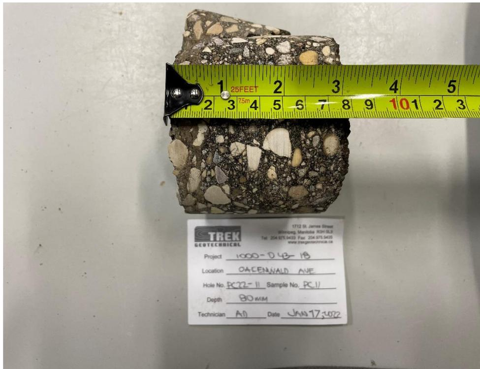
Photo 2: Pavement Core Sample at PC22-11
