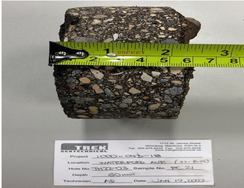
Photo 3: Pavement Core Sample at Test Hole TH22-03
