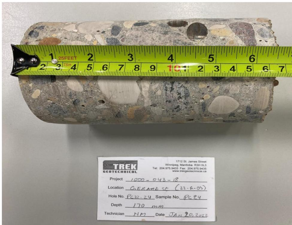
Photo 2: Pavement Core Sample at PC22-24
