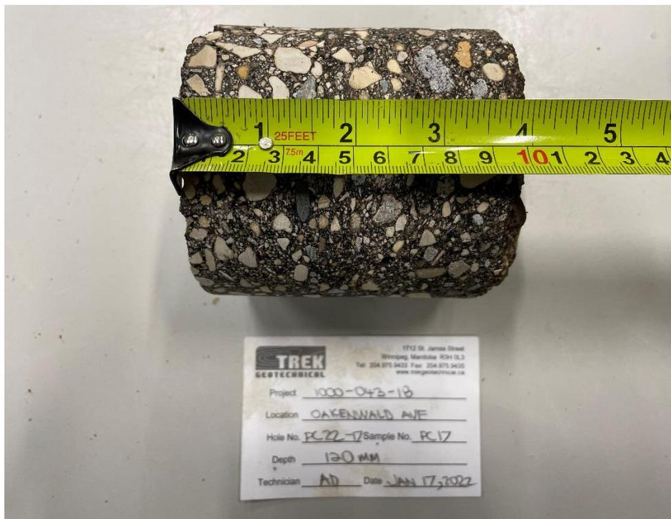
Photo 8: Pavement Core Sample at PC22-17
