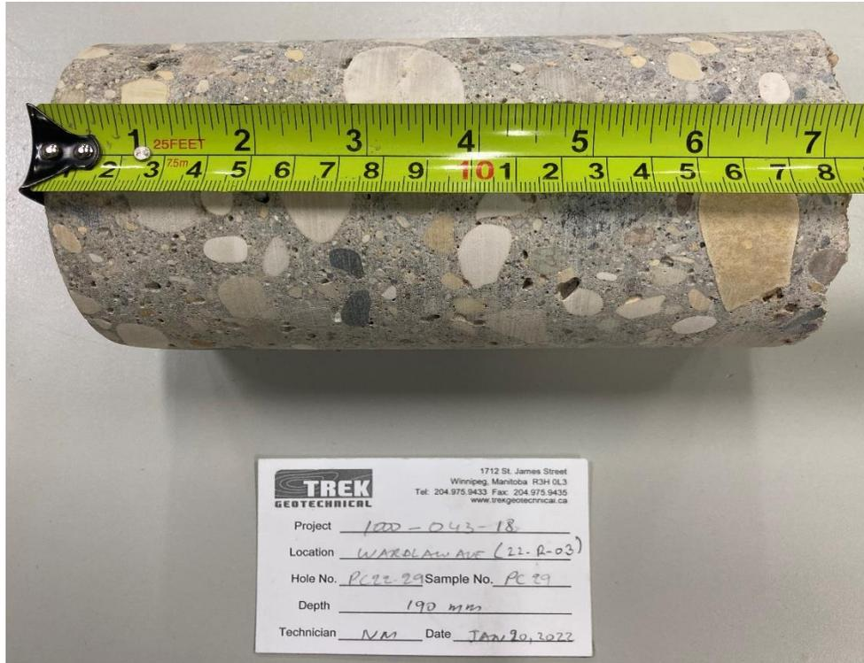
Photo 9: Pavement Core Sample at PC22-29
