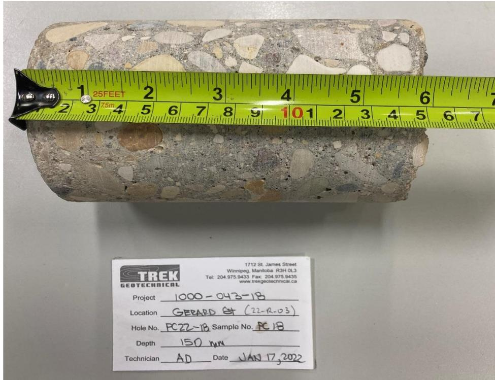
Photo 1: Pavement Core Sample at PC22-18
