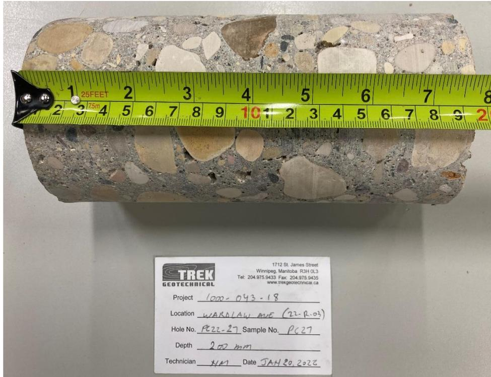
Photo 7: Pavement Core Sample at PC22-27
